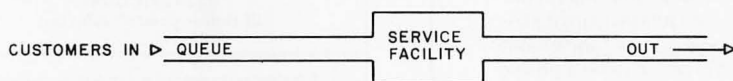
Figure 3: A single queue single facility system with one waiting line and one service area.
