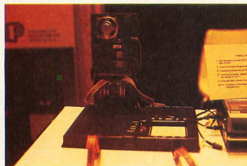
Photo 6: Color expansion board for the RCA Cosmac VIP computer. The board costs $89 and generates eight colors as well as musical tones.
