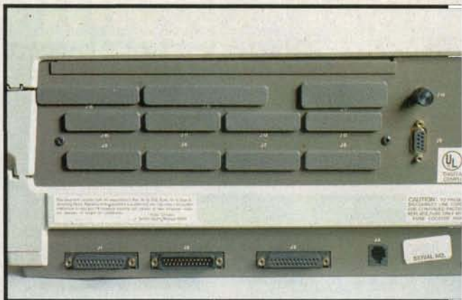
Photo 6: Part of the back panel of the Z-100. Along the bottom are two serial connectors (both male and female), a parallel printer port and a light-pen connector. On the upper right is a brightness control for the internal display, just above a connector for an RGB monitor. Note the wealth of cut-outs for optional connectors.
