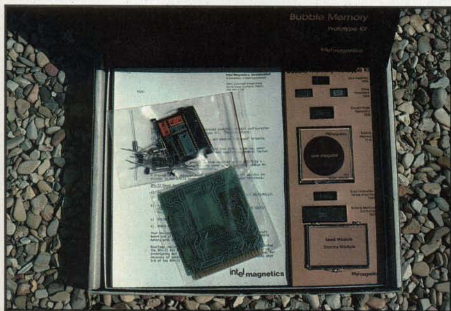
Photo 1: The Intel Magnetics Inc. BPK 72 Bubble-Memory Prototype Kit comes complete with a 4- by 4-inch PC board, all components, and extensive documentation. A simple interface and some software are all you need to build an S-100 disk emulator.
