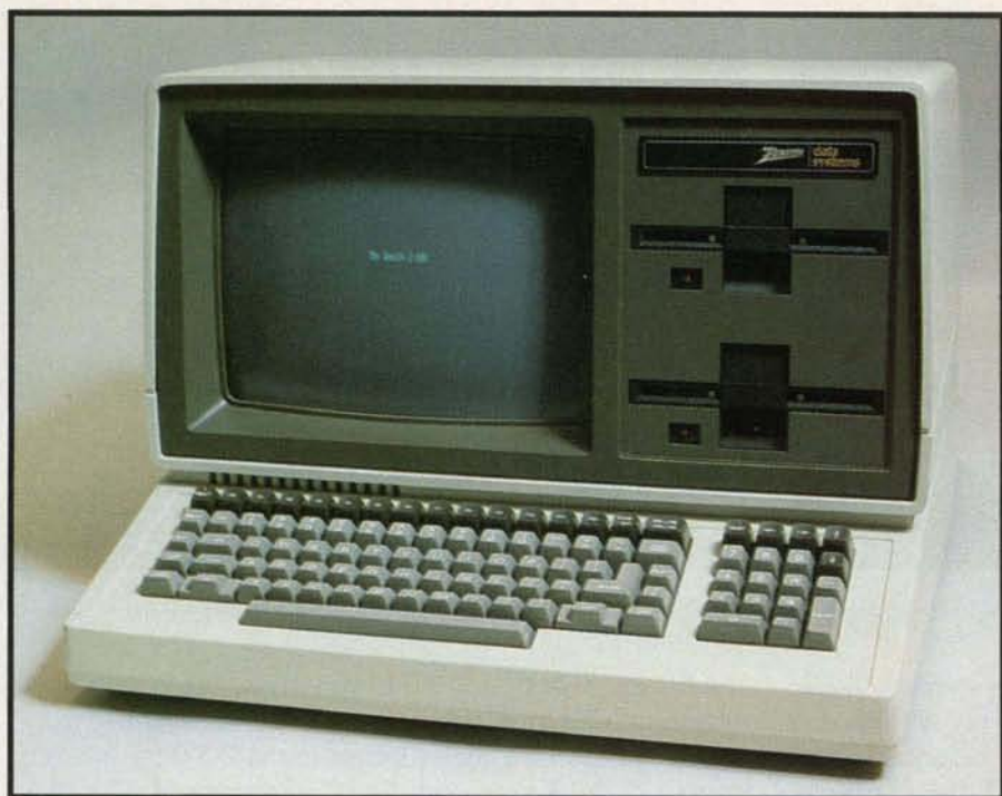
Photo 1: The Zenith Z-100. This version features a monochrome monitor in All-in-One style. In another configuration, the Low-Profile style, the monitor is in a separate enclosure and the disk drives are arranged horizontally above the keyboard. An RGB color monitor is available for both styles. Note that the keyboard has an IBM Selectric-style key layout, with a numeric keypad on the right and a row of function keys along the top.
