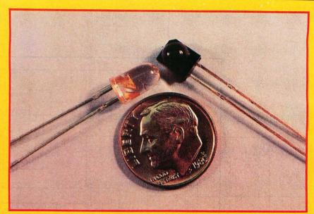
Photo 1: The TIL413 infrared-sensitive PIN photodiode (right) and the TIL39 infrared light-emitting diode (left).
