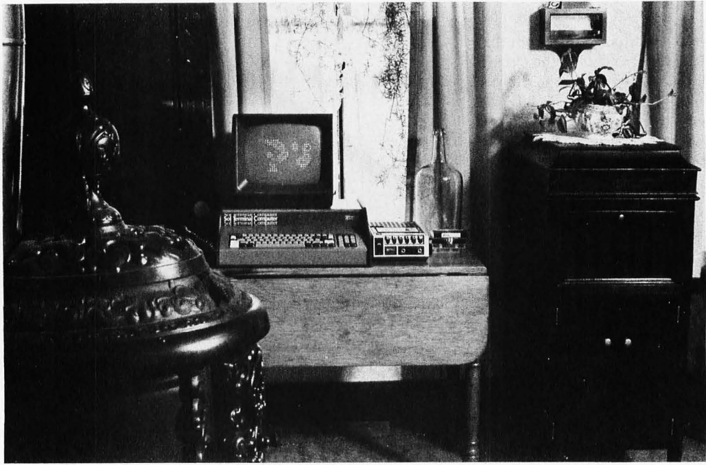
The SOL-20 in a New England parlor context, obviously enjoying life. The entire system fits on one table with a video monitor on top of the computer and an audio tape recorder for mass storage to the right.
