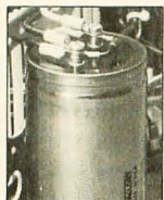
OVERSIZE CAPACITORS 280,000 uf FILTER CAPACITANCE -8V 43,000 uf FILTER CAPACITANCE ON EACH ± 16V dc.
