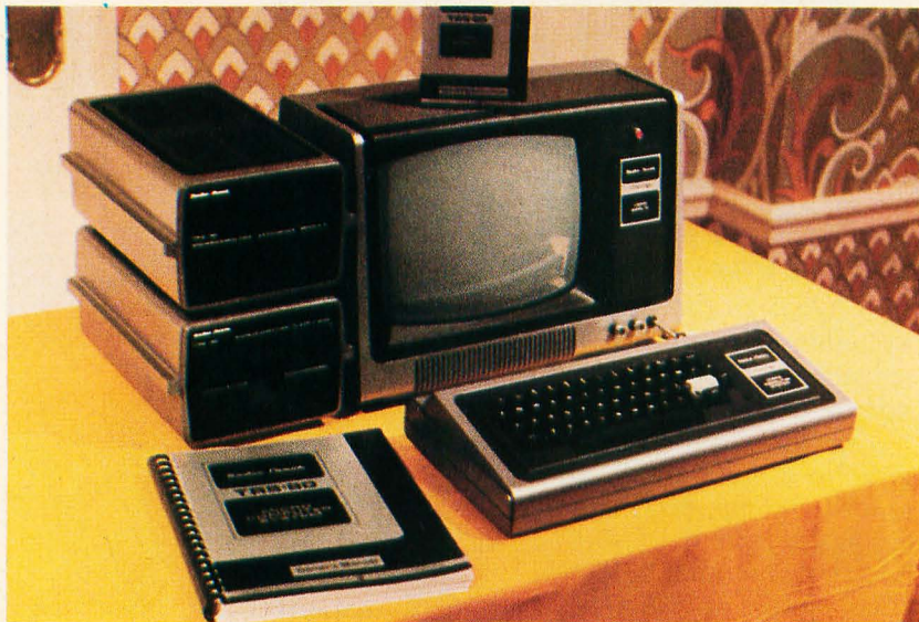
Photo 1: The New Radio Shack TRS-80 home computer system. Shown are the keyboard, video display monitor, instruction manual and prototypes of the upcoming memory expansion module and disk drive.
