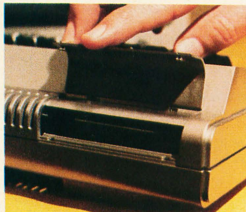
Photo 3: Rear view of the Radio Shack computer showing the 40 pin IO connector.
