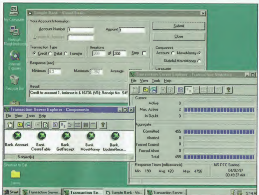
Microsoft Transaction Server Explorer monitors ActiveX controls and provides useful statistics about the transaction load on them.
