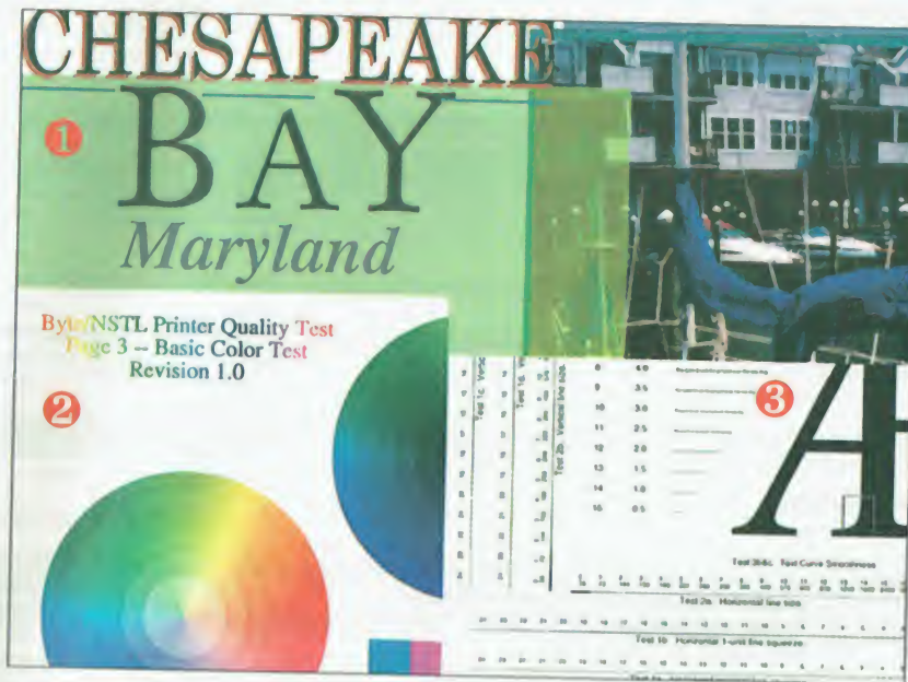
Among other pages, the NSTL Printer Quality Test has a color page with mixed content (1), color graphics (2), and text and fine lines (3).
