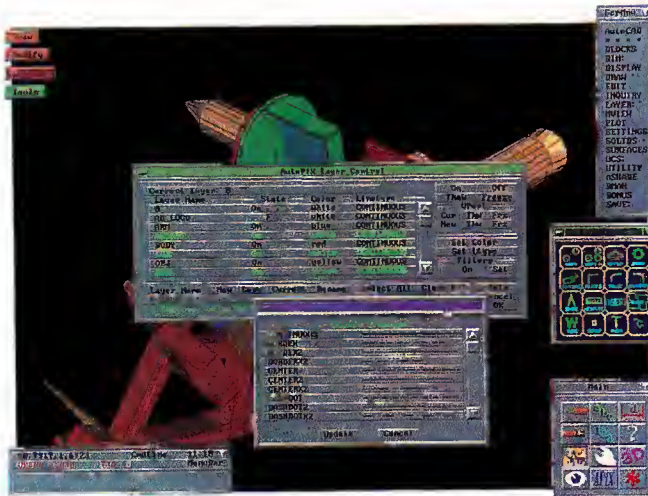
AutoPix displays AutoCAD's prompt area, screen menu, and pull-down menus in movable panels that you can resize and shrink into icons when not in use.
