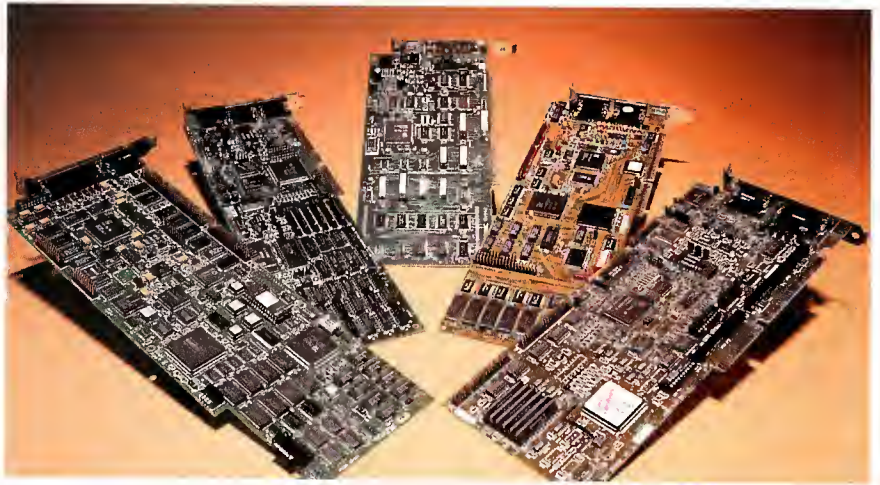
Hardware for pulling video into Windows (from left to right): the Matrox Marvel, VideoBlaster and VideoSpigot from Creative Labs, AITech's VideoSurge, and New Media Graphics' Super VideoWindows.
