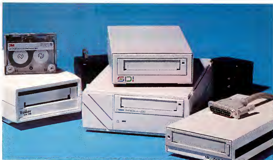
Portable tape drives connect to your PC through a standard printer port and provide tape backup-and-restore functions. Pass-through connections let you keep your printer connected at the same time. From left to right: Colorado Memory Systems' Jumbo Trakker 250, SDI's Model 250P (top), Iomega's Tape250, and Micro Solutions' Backpack tape drive. All except the Iomega Tape250 use an external power brick (the Trakker's is a bit large for portable use).
