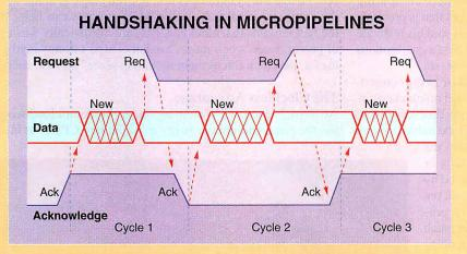
**Figure A:** The first phase of the bundled-data convention (red arrows) is initiated by the sender. The second phase, initiated by the receiver, is in green. The convention is said to be "bundled" because the request, acknowledge, and data lines must be treated together when factoring in circuit delays.
