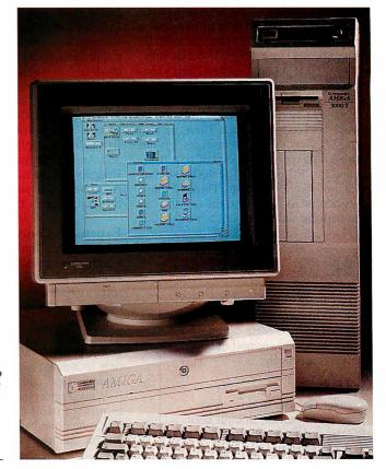
3000T), you can use an ordinary VGA monitor with the new models. The new video controller still supports optional genlock (video overlay) and all the old Amiga video modes. If your applications software gets confused, however, the 4000-040 can emulate an older graphics chip set.
