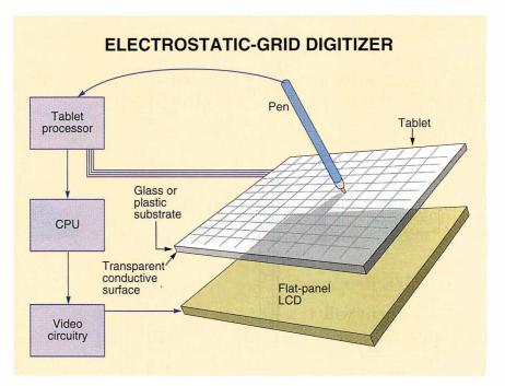
**Figure 2:** The tablet controller in an electrostatic-grid digitizer generates electrostatic signals across a wire grid on the tablet surface. A capacitive probe in the pen tip couples with the tablet and transmits received signals through a tether to the tablet controller, which calculates the pen's position.
