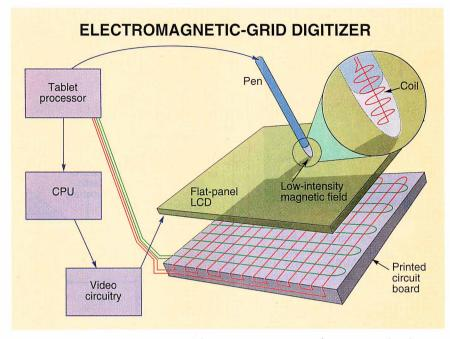
**Figure 1:** In an electromagnetic-grid digitizer, a continuous electromagnetic wire grid acts as an antenna on the tablet surface. When the pen approaches the surface, a wire coil inside the pen generates a low-intensity magnetic signal that induces a small voltage in some of the grid wires. The tablet processor then detects the voltage and translates it into x, y coordinates.
