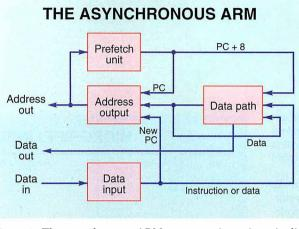
**Figure 1:** The asynchronous ARM processor is a micropipeline made up of smaller micropipelines. It takes data and instruction inputs and spits out addresses and data. PC stands for the "program counter."
