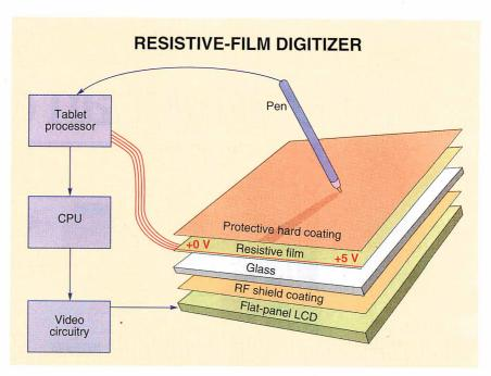
**Figure 3:** In the resistive-film design, an insulating glass surface is coated with a transparent, slightly resistive conductive coating. The tablet processor applies a 0-V AC current to one edge of the tablet and +5 V to the opposing side. Voltage ranges from 0 V to 5 V as the pen moves across the surface. The tablet controller calculates the pen's x position and then applies voltage to the top and bottom edges to determine the y value.
