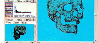
Adaptive screening software in the Digibot II automatically produces a greater number of points in an object that contains a sharp curve than in one that contains a gradual curve.
