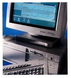
troller. Epson contends that this design, plus the 486's internal 8-KB cache, delivers high system performance without the considerable expense of a second-level cache.
