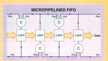
**Figure B:** Data moves through the pipeline in waves, depending on the state of the inputs at each stage. The bubbles on the acknowledge inputs of the Muller *C*-elements represent inverters.
