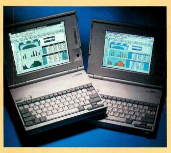
The Compaq LTE Lite 4/25C (right) uses Intel's new lowpower 486SL processor. The LTE Lite/25E features an eyegrabbing active-matrix display.
