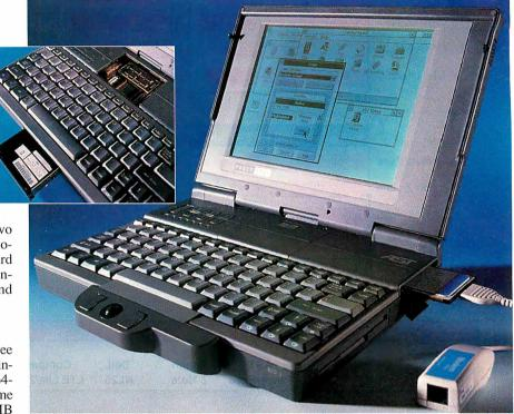
AST's new PowerExec notebook features PCMCIA support, a clip-on trackball, an upgradable screen, and (inset) a removable hard drive and an upgradable CPU.
