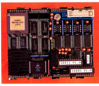
The adt164 is built around Burr-Brown's new CMOS converter, which allows the module to reach high speed with low power consumption.
