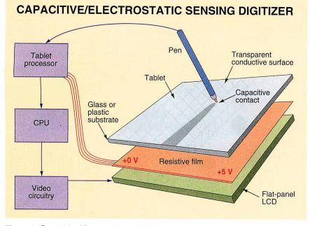
**Figure 4:** Capacitive/electrostatic technology uses a transparent substrate of glass that's coated on its underside with a sheet of a transparent conducting material. The 0-V and 5-V AC voltages, applied on opposite edges of the tablet, create an electrostatic field over the glass. A capacitive probe tip in the pen picks up this signal, which varies in strength over the tablet surface.
