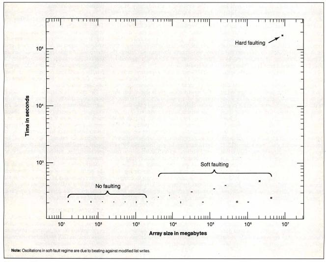
Figure 2: When a program tries to address memory outside the working set of directly addressable pages, execution time increases: slightly on a soft fault (memory found on the free list), and significantly on a hard fault (disk I/O required).
