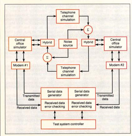
Figure A: This simplified block diagram shows the setup for testing each pair of modems.
