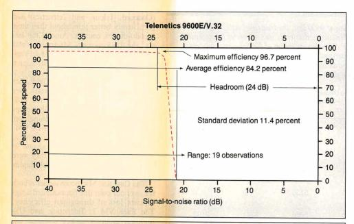
Figure 1a: The SNR Maps here and in figure 1b show that the Telenetics modem ran with greater efficiency than the Ven-Tel modem under typical line conditions. The Telenetics modem, though, showed a much narrower range of operation. Shown here are the raw test results for the Telenetics 9600E/V.32. a true V.32 modem, (In ideal performance, maximum and average efficiencies are high and close to one another, the standard deviation is a small value, and the range is a large value.)
