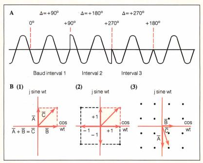
Figure A: A phase-modulated sinusoid. Figure B: (1) The sum of two vectors. (2) The sum of integer orthogonal components. (3) Amplitude scaling of orthogonal components.
