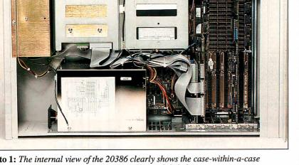
**Photo 1:** The internal view of the 20386 clearly shows the case-within-a-case construction that allows extra space for additional disk drives.
