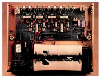
Photo 2: HAL in the prototype stage. The input jacks are arranged along the top; HAL's battery is near the bottom.
