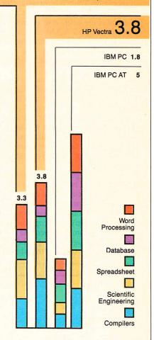
Indexes show relative performances; for all indexes, an 8-MHz IBM PC AT=1; graphs are based on indexes.
