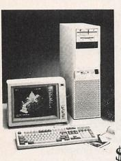
1 MB SIMM Module RAM 1.2 MB or 1.44MB Diskette Drive Chips & Technology 82C307 Cache High Speed 1:1 Dual Controller Enhanced 101 Tactile Keyboard 200W Power Supply **Tower Case** 80MB 28ms Hard Drive 16 Bit High Speed VGA Controller High Resolution VGA Monitor DOS 3.3 w/GW Basic 80386 Intel 25MHz CPU Chips & Technologies 386 Chipset Interleave/Page Mode 0 Wait Shadow RAM, Clock, Battery, AMI BIOS 8 I/O Expansion slots, EMS 4.0 support Expandable to 16MB on Motherboard Socket for 287/387/Weitek
