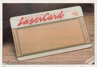
**Photo 9:** Drexler's wallet-size LaserCard contains a 35-mm strip that can permanently store several megabytes of data. Its current use is storing medical and insurance data.
