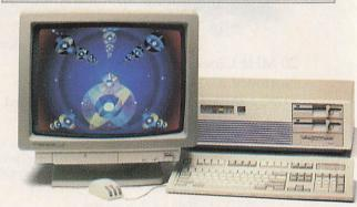
25 MHz Clock, Zero Wait Operation Norton SI 28.2 • Landmark Speed 33.6MHz Norton SI 31.6 • Landmark Speed 43.5 w/Cache 1024K, 1.2MB or 1.44MB Drive, 101-Keyboard Standard System Features:
