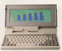
T1000: 6.4 lbs, 4.77MHz 80C88, 512KB RAM expandable to 1.2MB. MS-DOS in ROM, 720KB 3<sup>1</sup>/<sub>2</sub>" diskette drive. Built-in RGB, parallel, serial and external drive ports.
