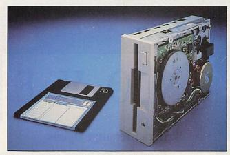
**Photo 8:** A "floptical" disk is a 3½-inch floppy disk that uses optical and magnetic recording technologies and can hold 20 to 25 megabytes.
