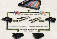
PowerCache 4 is the first PC to fully utilize 128-bit burst mode and a "read and writeback" 128KB cache design, providing better than zero wait state performance as compared to the i386.
