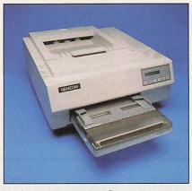
An 8-page-per-minute Canon engine drives the Genicom 6142 laser printer.
