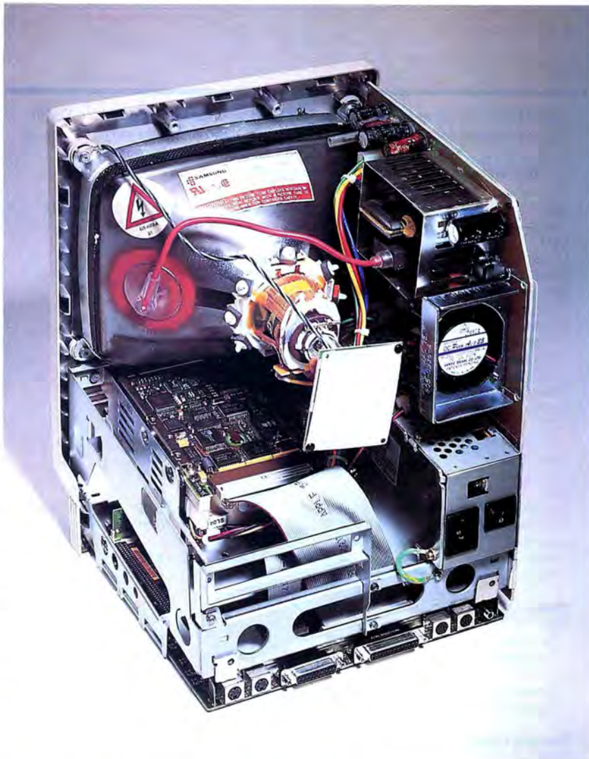
Photo 2a: The cramped insides of the Mac SE/30.
