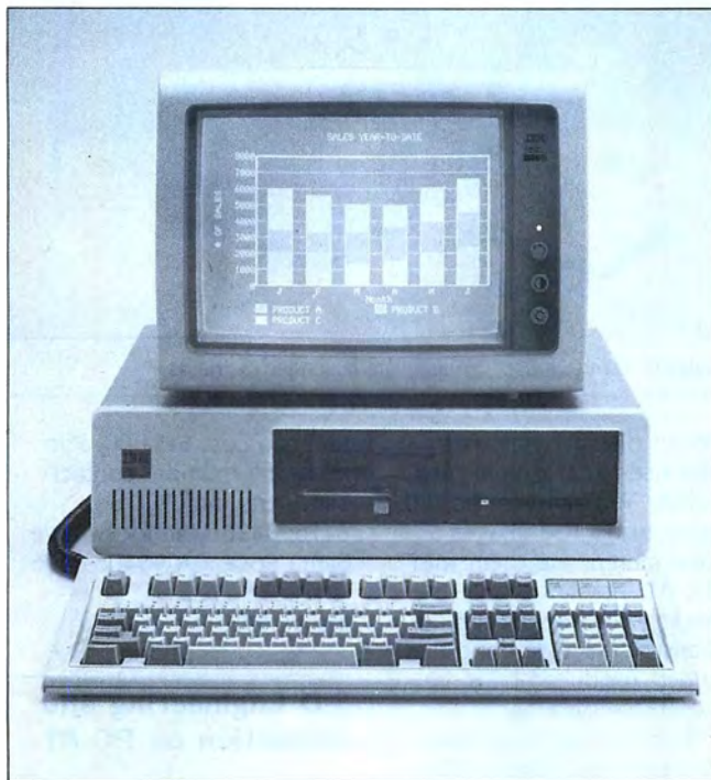
IBM's PC XT Model 286 runs on a 6-MHz 80286.
