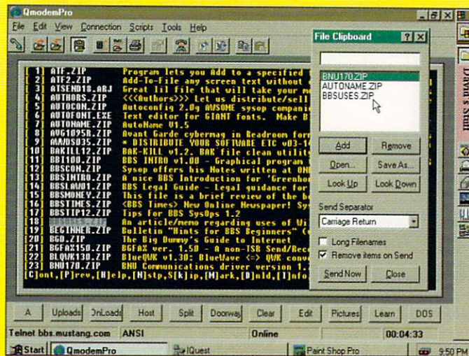
The File Clipboard is a great place to store a list of files you want to download. Just double click the file name on screen to select it, then drag it into the File Clipboard.
