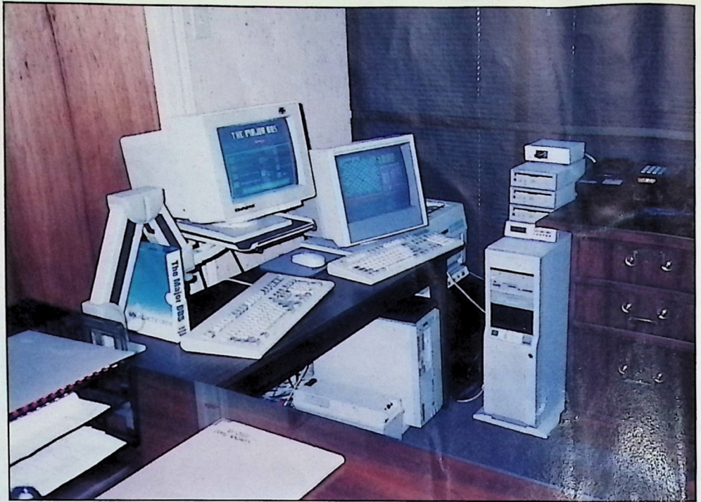
Emerald Palace Setup includes, 486/50,3 CDRoms, 56kbps x.25 Modem, 2 Galactiboxes Housing 32 Internal Modems and a 386/25 Development Machine.
